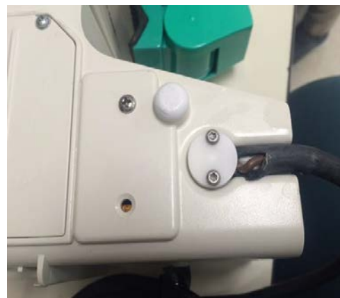
Frayed power cord on pump
