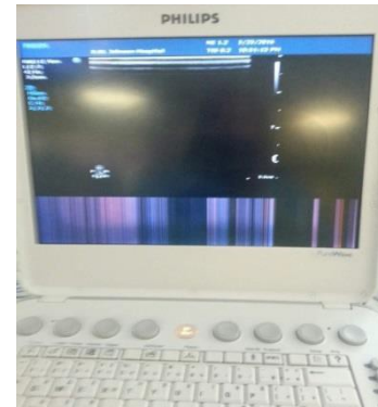
Broken LCD on ultrasound
